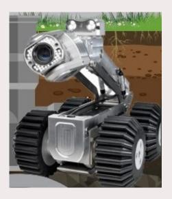
Video inspection technology for wastewater and storm sewer systems can help you identify and prioritize maintenance issues, while improving service and reducing emergency maintenance costs.
